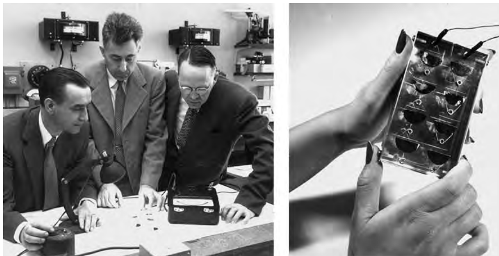
Figure 1.11 The inventors of the first “real” solar cell: Chapin, Fuller and Pearson. The right hand figure shows the first “solar module” in the world, a mini module of 8 solar cells (Courtesy of AT&T Archives and History Center)
