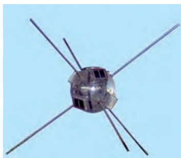
Figure 1.12 View of the Vanguard 1 satellite: Because of the diameter of 16 cm it was also called “Grapefruit” (photo: NASA)
